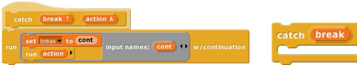
The upvar **break** has as its value a continuation that can be called from anywhere in the program to jump immediately to whatever comes after the **catch** block in its script. Here's an example with two nested invocations of **catch**, with the upvar renamed in the outer one:
